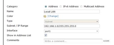
Create a remote LAN address. Set **Type** to **Subnet**, **Subnet/IP Range** to the Branch subnet, and **Interface** to the VPN Phase 1.
