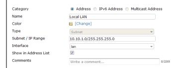
Create a remote LAN address. Set **Type** to **Subnet**, **Subnet/IP Range** to the HQ subnet, and **Interface** to the VPN Phase 1.
