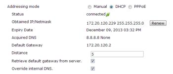
If the IP address seems incorrect or missing, select **Renew** to renew the lease and get a new IP configuration from your ISP. If you cannot get a valid IP address this way, the FortiGate unit cannot communicate with the ISP's DHCP server.
